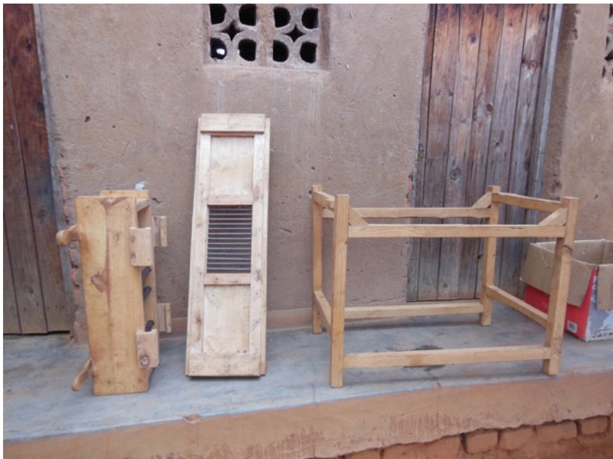
A partially disassembled wooden sheller in Dedza
